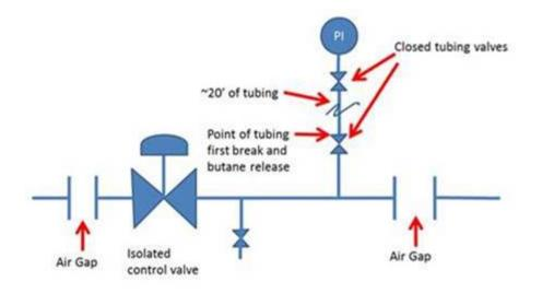
Would your company consider this a PSE? Does the fact the section of piping the tubing was connected to had been physically isolated from the process (with air-gap) rather than just isolated make this scenario different from Example 28 in <u>API RP 754 2nd edition or Example 31 from API's February 2nd,</u> 2012 RP 754 Question and Answer webpage?
